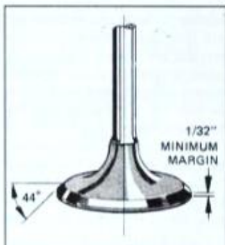
Exhaust valves should have margins of at least 1/32 in. after grinding to minimize risk of burning. Intake valve margins should not be less than 1/64 in.
