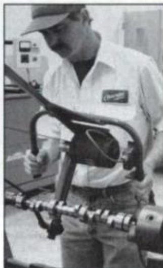
Camshaft bearing journals are getting same polishing treatment as crankshaft. Abrasive belt runs against journal as cam rotates between centers.
