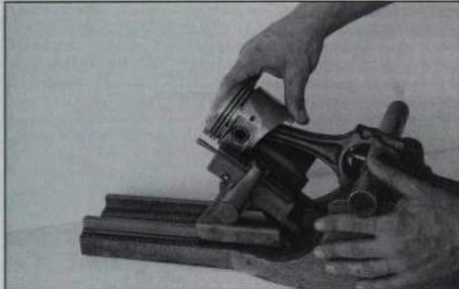
Placed in checking fixture, piston is rocked back and forth while indicator mark is observed. If it moves, rod is twisted or bent. If bend or twist is minor, rod can be straightened and reused.
