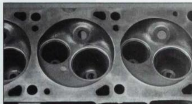
Dark bands are valve seats. After 45° seat is cut, seats are blued so they'll be contrasted from 30° and 60° cuts to ease measuring. Narrow strip of paper with tick marks, divider and 6-inch scale is all that's needed for measuring seats. Seat widths shown are 0.090 in. and 0.060 in. for exhausts and intakes, respectively.
