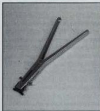
Ring expander makes installing compression rings much easier and greatly reduces risk of breakage. Inexpensive expander adjusts to spread needed to install ring.
