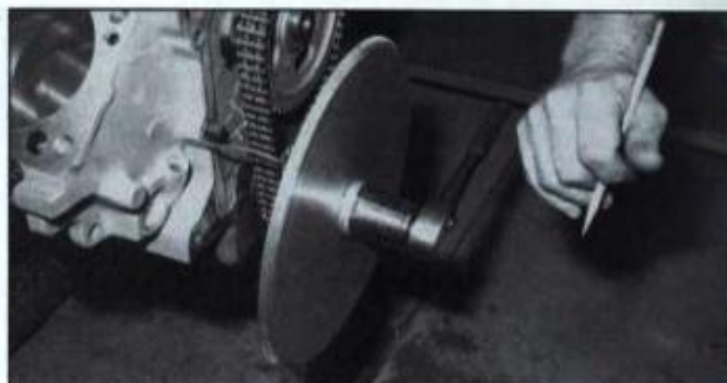
Available from camshaft manufacturers and high performance engine parts suppliers, a degree wheel is a must for checking camshaft against the manufacturer's specifications. Directions are printed on wheel.
