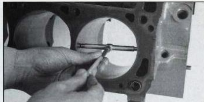
Telescoping gauge is locked to hold plungers in position at a specific location, locked in position, withdrawn from bore, then measured with outside micrometers to determine bore size. Subtract unworn bore size from that having maximum wear to determine taper.
