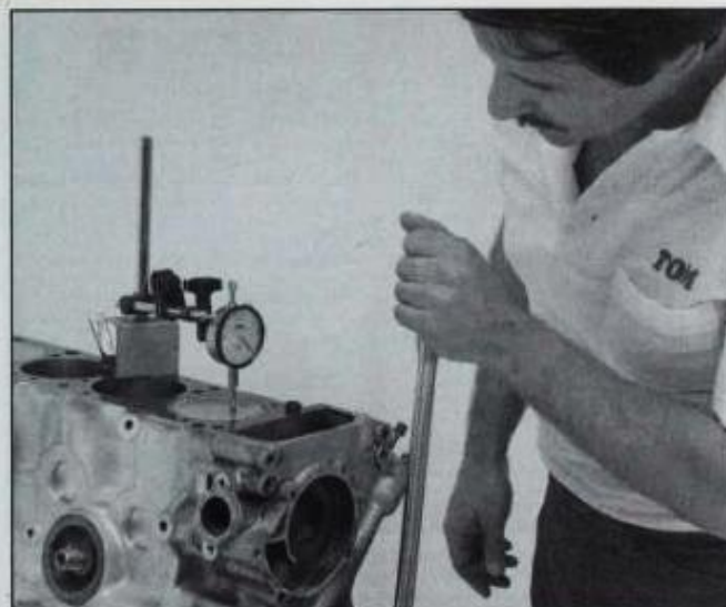
Dial indicator can be used to check crankshaft end-play, flywheel warpage, crankshaft runout and camshaft IRL. Magnetic base works well on flat magnetic surfaces; bolt-on stand is used on irregular surfaces or non-magnetic components such as aluminum cylinder heads. Indicator is being used to find TDC.
