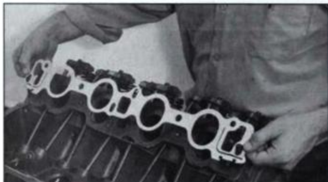
Separate manifold-to-cylinder head gasket is fitted to head. Apply bead of RTV sealer around water passages.
