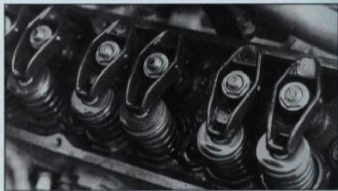
On stud-mounted rocker arms used with solid lifters, adjustment can be maintained for longer intervals by installing sheet-metal PAL nuts or Tinnerman nuts on top of standard locknuts.
