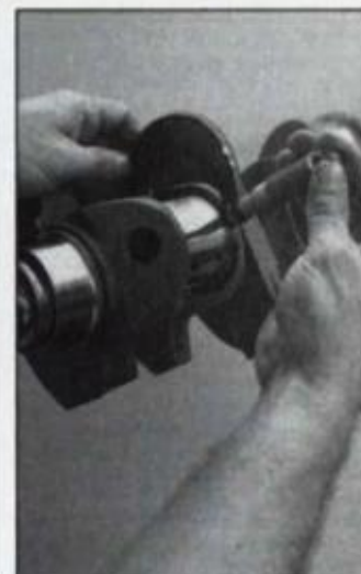
Front throw is measured for out-of-roundness. Compare measurements made 90° to each other in the same plane. I like to keep differences between these two measurements less than 0.001 in. (0.02mm) before regrounding crankshaft. Measure all bearing journals.
