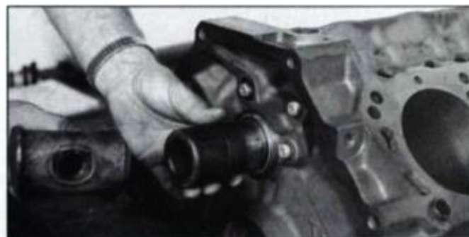
Cup-type cam plug is similar to core plug but has shorter flanges. After applying sealer to flanges, install in a manner similar to how you installed core plugs. Plug that has no flange installs with convex—open-side in. To secure it, drive center in until flat.
