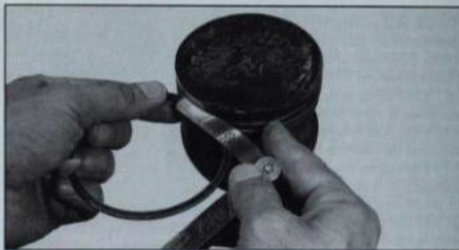
Check ring-groove width with ring and feeler gauge. Ideal side clearance is 0.0025 in. (0.06mm) and absolute maximum is 0.006 in. (0.15mm).
