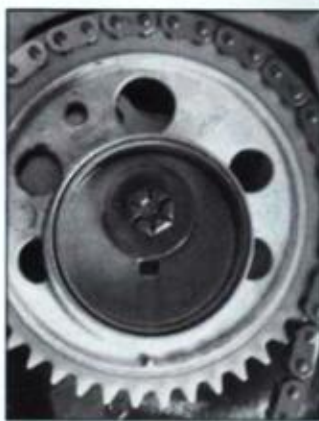
Secure cam sprocket with bolt and washer. If your engine uses a separate fuel-pump eccentric, install it too. Note sprocket timing marks.
