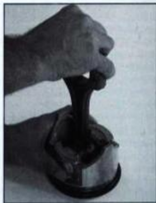
Check piston pin bore wear by grasping piston and rod as shown and rocking rod from side to side, then twisting rod. Place finger and thumb over end of pin. If you feel any movement at pin, piston should be replaced. Pin-to-bore clearance should be about 0.0005 in. (0.01mm).
