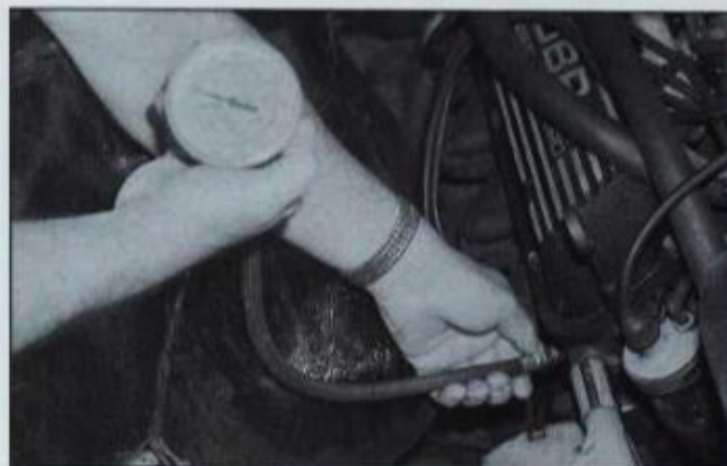
In preparation of doing compression test remove all spark plugs. Disable ignition, prop throttle and choke plates open then spin engine over four times on the compression stroke for each cylinder. Pressure of worst cylinder should be no less than 75% of best one.
