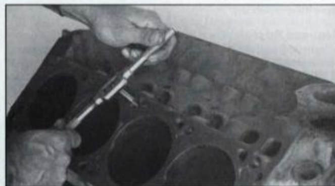
Using correct tap, chase each threaded hole in block. Clean threads will help ensure bolt are torqued correctly during assembly. Remove debris and liquid from bolt holes with compressed air.
