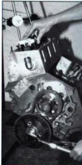
Allen Johnson uses valves installed with light springs, lifters and pushrods to check valve-to-piston clearance. Dial indicator with plunger set square against spring retainer and parallel to valve stem is used to read valve movement and thus valve clearance. At each 2° increment of crankshaft rotation between 20° before and after TDC, valve is pushed open until it touches piston. Clearance is read directly from dial indicator.
