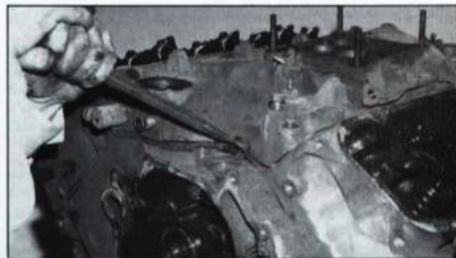
Intake manifolds can be ornery. Before you resort to breaking loose manifold as shown, double-check that you've removed all bolts. Be very careful not to damage gasket surfaces, particularly head-to-manifold surfaces.
