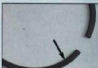
Always read directions that accompany pistons rings. Mark on ring indicates top of ring, or side that installs up.
