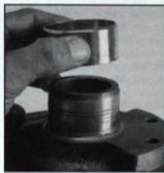
Good news! If damper seal surface is badly grooved or otherwise damaged, you don't have to buy another damper. This thin metal sleeve from Fo-Pro installs over damaged seal surface.
