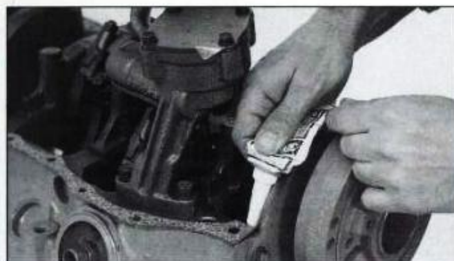
Neoprene oil pan end seals in this engine must be worked into grooves in front cover and rear main. RTV sealer is used at joints between front and rear oil-pan end seals and oil-pan-rail gaskets. If yours is a one-piece oil-pan gasket, this is one operation you don't have to be concerned with. Just fit gasket to bottom of engine.
