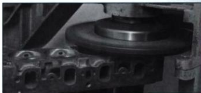
Resurfacing cylinder head. If more than 0.020 in. is removed from head that goes on a V-type engine, bottom and sides of intake manifold should be resurfaced to maintain intake-port alignment. There are other considerations: Compression may be raised to too-high a level and shorter pushrods may be needed if rocker arms are not adjustable. Valve-to-piston clearance will also be reduced.
