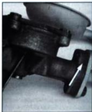
Critical to lubrication system operation is oil pump pickup. Clean screen, then attach pickup to pump. This one bolts on. Crack through flange at bolt hole (arrow) in new pump didn't appear until pickup was bolted on. Disaster could have resulted if crack wasn't discovered, so never stop looking.
