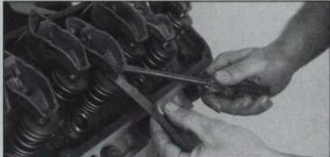
Check valve tip-to-rocker arm clearance of non-adjustable valvetrain after prying between valve retainer and rocker arm to bleed down lifter.
