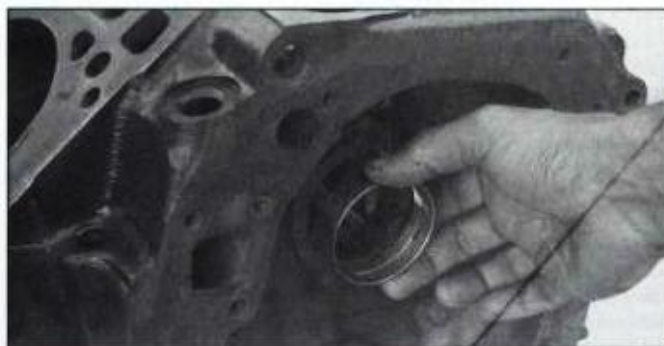
This front cam bearing has two holes and a groove in between. One is an oil supply hole and the other is for supplying oil to distributor shaft bore. Always check bearings as shown before installing them.
