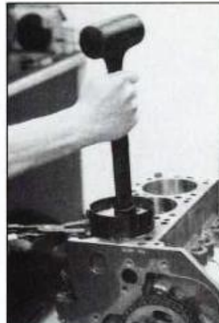
With block positioned so bore is vertical, crankpin at BDC and rings compressed, insert rod and piston into bore. Check orientation of piston and rod—piston arrow, notch or whatever to front and rod number to the correct side. With compressor hard against block deck, push or lightly tap piston into bore with hammer handle. If you feel any resistance, STOP! Pull piston out and start over by recompressing rings.
