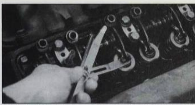
A solid lifter valvetrain requires some lash, or clearance. This is characterized by a light clicking noise. Excess lash results in a clattering noise; too little clearance and the valve may not close fully.
