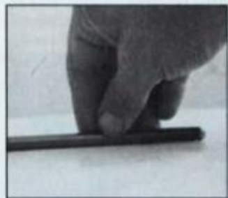
Check pushrods for straightness by rolling on a flat surface. With a light on the opposite side, look under each pushrod as you roll it. If you suspect pushrod is bent, check it with a 0.008-in. (0.20mm) feeler gauge. If the gauge fits, don't try to straighten pushrod. Replace it.
