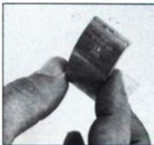
Stamped into back of bearing insert is part number and relative journal size. Bearings will be standard (STD) like this one, or undersize as indicated by .010, .020, etc.
