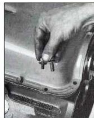
Take a last look at bottom end before you install oil pan. If all is OK, carefully set oil pan on gaskets, being careful not to move them out of place. Install and snug bolts. This pan uses larger bolts at four corners. Don't overtighten bolts and dimple pan flange.
