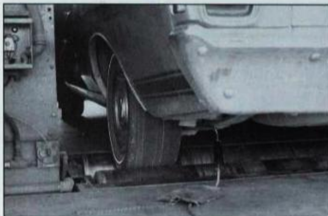
Performance tuning is best done with engine under load. Chassis dyno allows this to be done in shop where all engine functions can be monitored. Exhaust probe picks up samples that are routed to gas analyzer.
