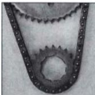
Crank sprocket's nine keyways are for timing camshaft straight up as well as four advanced and four retarded positions in 2° increments. Maximum advance and retard is 8°. Cam timing for best performance is found through a combination of dynamometer and track testing.
