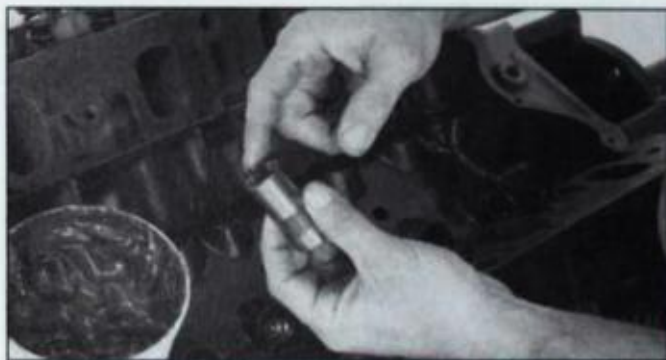
If you're reusing cam and lifters, install lifters in their original bores. If you've lost track of their original order, install new lifters to avoid wiping out a camshaft.
