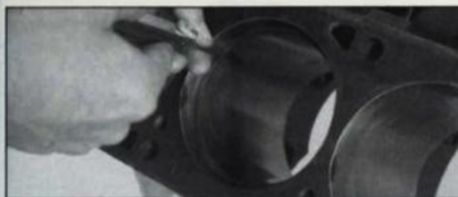
Check ring end gap with feeler gauges. A little too much ring gap is not a problem, but too little can be disastrous. If ring ends butt because of inadequate end gap, cylinder scoring will likely result.
