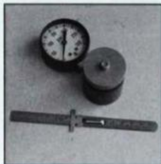
Spring testers used in machine shops are very expensive, however this one is relatively inexpensive. All you'll need is a bench vise and 6-inch scale. Gauge reads out directly in pounds.
