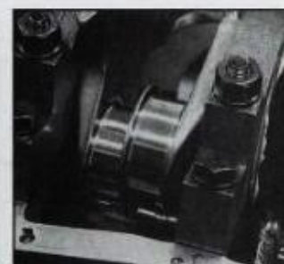
Be sure to tighten main cap bolts to the correct specifications, both torque and, in some cases, sequence. If four-bolt main caps are used, outboard bolts are usually torqued to a lesser amount. With cross-bolted caps, spacers between block and caps fit with zero clearance.
