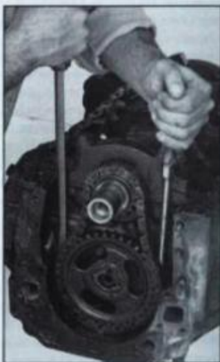
Remove timing set by inching sprockets off together a little at a time. Screwdrivers used as shown usually work. If not, a puller on cam sprocket or crank sprocket may be required to get sprocket to budge.
