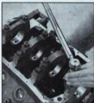
Torquing main bearing cap bolts in place is critical before honing. Force from bolts actually distorts bores ever so slightly, but enough to show up as uneven bore wear if caps are not in place during honing.
