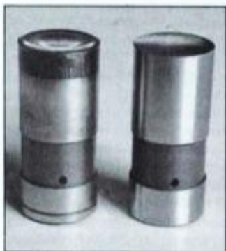
Badly worn lifter compared to new one; worn lifter foot exhibits a concave wear pattern. Lifter foot should be convex—raised in center.
