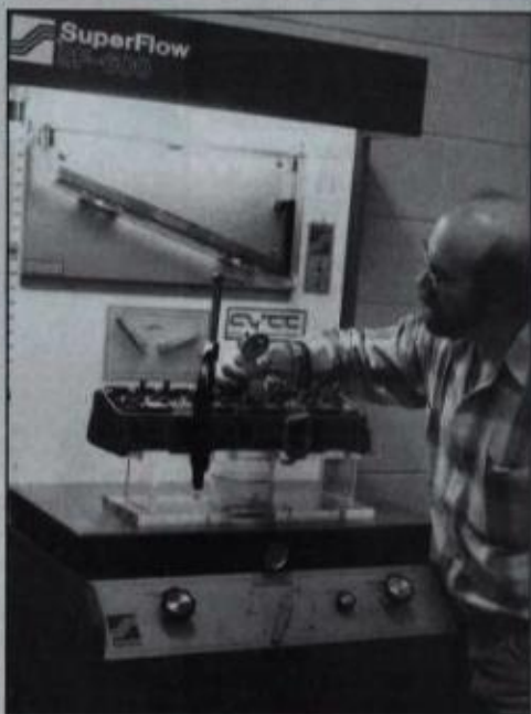
Only way to determine how much cylinder head flows is by testing on flow bench. Flow of ports is checked after making small modifications.
