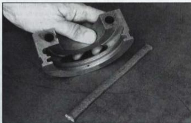
Pointed pin in rear main cap prevents rope seal from spinning in groove. If you will be installing a split lip seal, drive out pin from the back side of the cap using a 3/32-in. or smaller punch. Fill hole with silicone sealer to prevent oil from leaking out hole.
