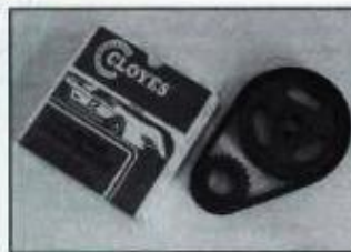
Roller timing-chain set has three keyways in crankshaft sprocket. This allows cam to be timed as designed by cam manufacturer, advanced 4° for more lower-rpm torque or retarded 4° for higher-rpm operation.
