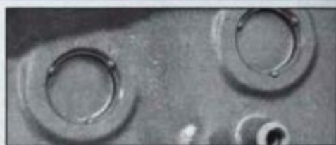
Recess pin core plugs so they stay put. Small brad-type rivets can be purchased at most fastener supply stores. Drill three holes square to chamfer at edge of each plug. Hole should be slightly smaller than rivet. Rivet heads should overlap plug flange. Drive in rivets to secure plugs.
