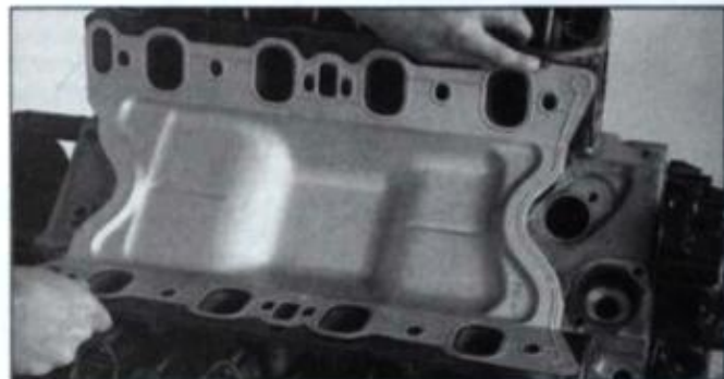
This V-8 uses one-piece metal-shim gasket/baffle under intake manifold.
