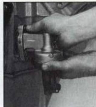
To make installation of mechanical fuel pump easier, turn crank until fuel pump eccentric is at lowest position. Apply RTV sealer to both sides of gasket.
