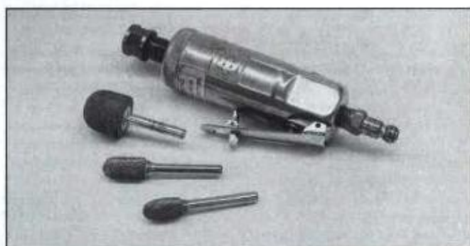
Pneumatic die grinder with assorted carbide burs, abrasive stones and paper rolls are a must if you intend to make serious cylinder head modifications.
