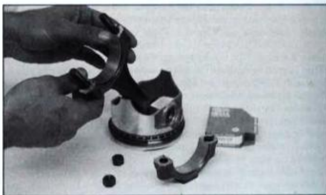
After wiping off bearing inserts and bearing bore in rod and cap with paper towel, install bearing inserts. If there is an oil hole in top bearing insert, check that it aligns with hole in the rod.
