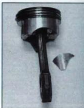
Sometimes broken skirt is evident, sometimes not. It may just be collapsed. Either condition is reason to replace piston.
