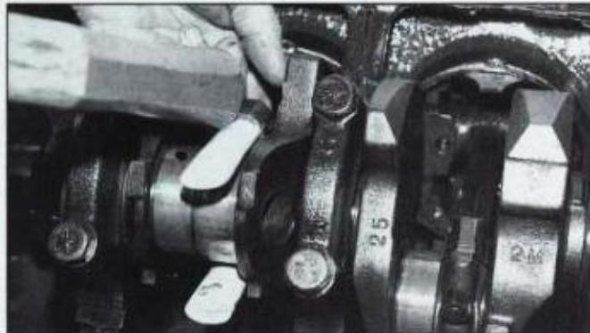
Use hammer handle or wood dowel to push against rod or underside of piston with one hand and catch it with free hand. Don't let connecting rod bang against bore.
