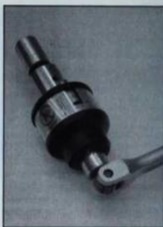
Installed between breaker bar and socket, when preset torque of sensor is reached it buzzes. If you must have all the "bells and whistles," torque sensor is available from Snap-on.
