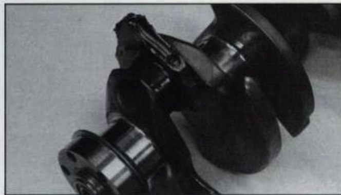
This engine experienced catastrophic failure at high rpm as evidenced by broken connecting rod and blue bearing journal. A crankshaft must be inspected for journal damage, cracks and straightness before it's declared OK for reuse.
