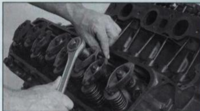
While cylinder is on TDC, rocker-arm nut is tightened to adjust valve. If rocker arm is adjustable with hydraulic lifters, rotate nut 1/2 to 3/4 turn after slack is taken up in pushrod, but before lifter plunger moves. Positive stop nut is simply tightened to spec, but it should not bottom lifter plunger.
