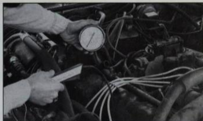
Vacuum gauge tells a lot about engine condition. Low vacuum—less than 15 in.Hg with street-cammed engine—usually indicates engine is in need of a rebuild. It can also be caused by retarded timing. Fluctuating needle is caused by a weak cylinder, typically from a misfiring plug, valvetrain problem or low compression in one cylinder.
