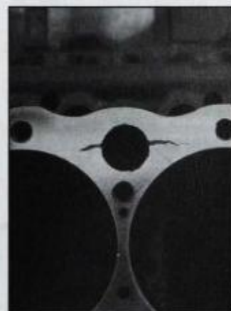
Dye penetrate is applied to area that's being checked for cracks after it's thoroughly cleaned. After cleaning again, developer is sprayed on area. Cracks show up as jagged red lines as dye bleeds through flat-white developer.
