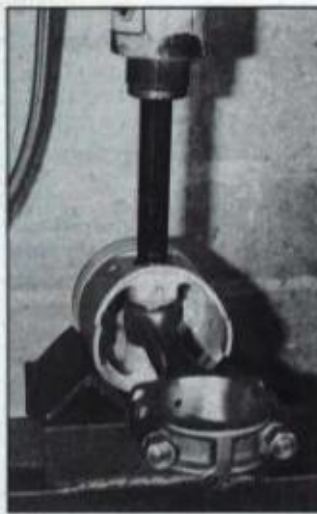
Disassembling piston and connecting rod with pressed-in pin requires a hydraulic press and mandrels. Never drive out wrist pin with a punch and hammer.
