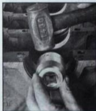
Brass hammer and large diameter cylinder like this socket are used to force rope seal into groove. Seal for cap was first installed in block to shape it, then removed and installed in cap. Work seal into groove, then trim ends flush with cap or block with a sharp knife or razor blade.
