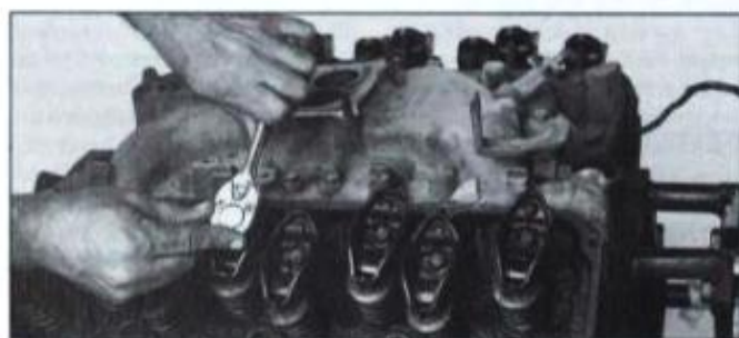
Remove individual rocker arms by first removing each hold-down nut or bolt. Regardless of valve-train setup, all parts must be kept in order and together so they can be installed as they came apart at assembly time. Machined parts that wear together must be kept together.
