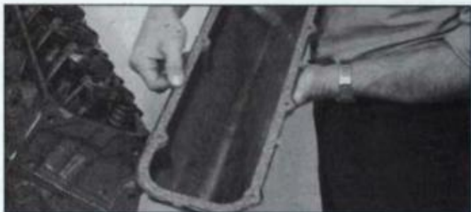
Fit gaskets to valve-cover flanges. Tabs on this cork gaskets snap into notches at edge of valve-cover flange. If holding gaskets in position is a problem, use small dabs of weatherstrip adhesive on flange. When installing valve cover be careful not to overtighten bolts.
