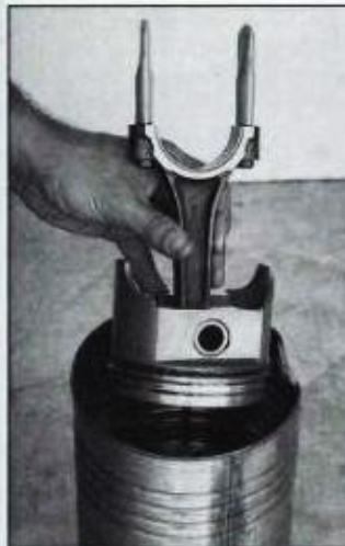
To pre-oil piston, immerse it in can so oil is over rings and piston pin. Rock connecting rod back and forth to work oil between pin and bore. Oil the rod bearing inserts and install rod bolt sleeves.
