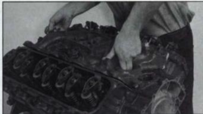
Be careful when installing intake manifold on a V-type engine. It's too easy to move gaskets out of position. Result will either be an oil leak or a huge vacuum leak and excess oil consumption.
