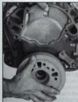
After installing gasket(s) to cover with sealer and applying sealer to block, fit cover to block. If cover is not positioned to block with dowels, loosely install bolts and center cover to crankshaft by installing damper. Tighten front-cover bolts.
