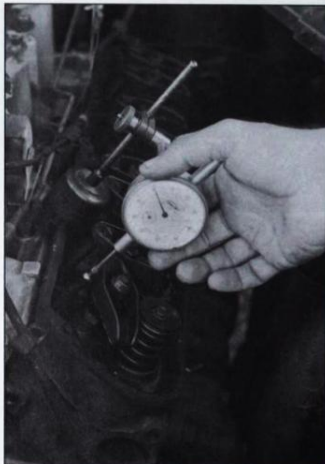
Lobe lift is measured directly with dial-indicator plunger tip positioned against pushrod tip. Zero indicator when lifter is on lobe base circle, then rotate engine slowly until maximum reading is obtained. This figure is lobe lift.
