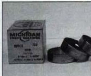
Check that cam bearings are the ones for your engine. Cross-check bearing part numbers to list on slip of paper in or on box, as is the case here.
