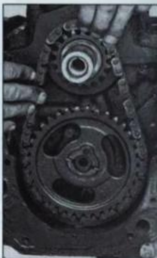
Chain hadn't jumped timing, but it wasn't far from doing so. Jumped timing frequently occurs when engine kicks back from dieseling or a backfire, advancing valve and ignition timing.
