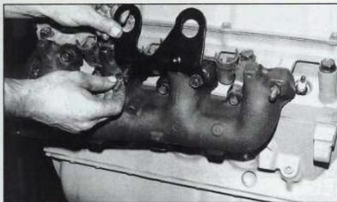
Check exhaust manifold for cracks. A good welder can make the repair. Smooth mounting faces with a large flat file. Replace header-pipe mounting studs if they are in bad shape.
