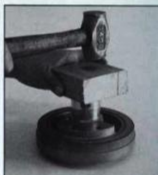
Apply RTV to the sleeve ID and drive it over original seal surface until it bottoms. Use a wood block between sleeve and hammer. Damper will be like new.
