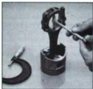
Cap is installed and bolts or nuts are torqued to spec in rod vise prior to measuring and resizing. Telescopic gauge is set in line with rod bore, the direction that cap distortion occurs to give an oversize condition.
