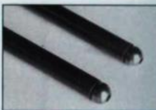
Wear at rocker arm end of pushrod extends farther around ball (top) than at lifter end. If you are installing new rocker arms or didn't keep pushrods or rocker arms in order, swap pushrods end for end.
