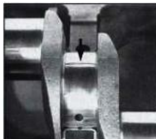
Double-check main bearing oil clearance with Plastigage. With crankshaft in place on dry bearings, lay strip of Plastigage the full length of the dry bearing journal, then install bearing cap. A very light film of oil can be applied to bearing in cap to keep Plastigage from sticking to bearing. Torque bolts to specification. Don't turn crankshaft. Carefully remove cap with bearings and check width of squeezed Plastigage with scale printed on edge of sleeve. Width corresponds directly to bearing oil clearance.
