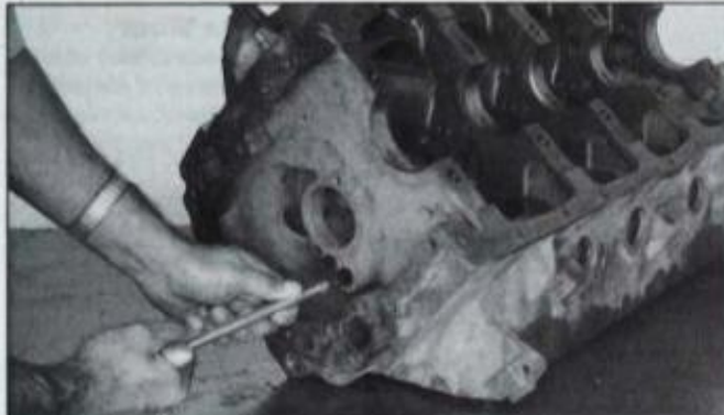
Following steam cleaning run a gun-bore brush through oil galleries to loosen stubborn deposits. Brush should fit tightly in passage. If brush handle is not long enough to reach to opposite end of passage, do one end, then run brush in from opposite end of block.
