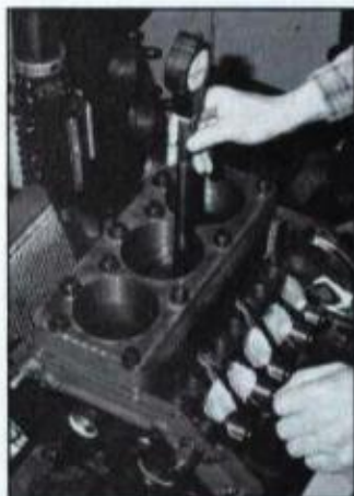
Deck plates are installed to simulate bolted-on heads. As with main caps, head bolts also distort bores. Unlike cylinder heads, deck plates allow access to cylinder bores for honing. Cross-hatch is restored to bores in freshening-up process between races. Minimum amount of material is removed from bores.
