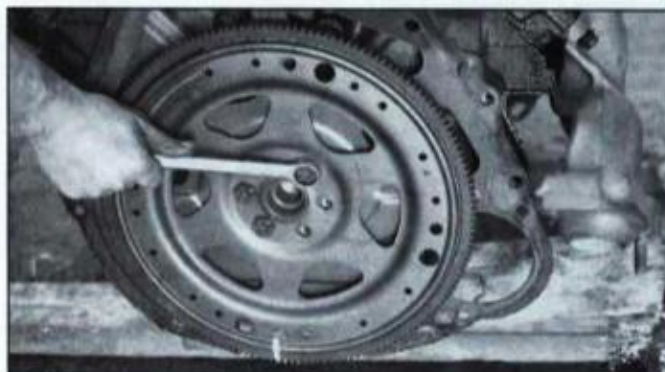
Remove flexplate or flywheel bolts with engine secured so it doesn't roll over. If you don't have an impact wrench, strike wrench with soft mallet to break loose bolts.
