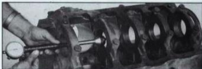
For maximum accuracy, bearings are installed in block without crankshaft, then ID is measured with dial bore gauge. Difference between bearing journal diameter and this measurement is oil clearance.
