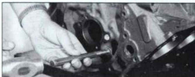
Cup-type oil gallery plug is driven in with punch. Punch should not fit tightly in plug, otherwise flange will collapse on punch as plug goes in. Seal plug and drive in just below hole opening. Secure plug by staking flange in three places with small chisel.
