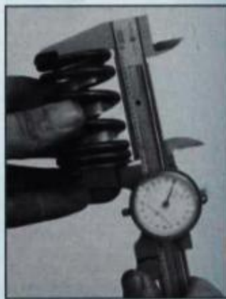
Two quick ways of determining whether a valve spring needs shimming and/or replacing. First, spring should be square. One shown is being checked with a carpenter's framing square. A valve spring should lean no more than 1/16 in. at the top. Check free height too. If heights vary from each other as much as these two check their load, or pressure, at installed height. Final check is to measure free height directly. Note flat wound wire inside spring. It's a damper.
