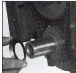
Fuel-pump eccentric prevents front crankshaft seal from being flooded with oil. It goes on before front cover and damper. Don't forget it or front seal will leak.
