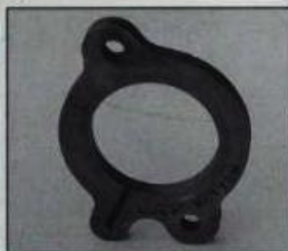
Cam thrust plates must sometimes be oriented in a specific direction and positioned to front face of block as is the case here. It routes oil from front cam bearing to distributor-shaft oil gallery.
