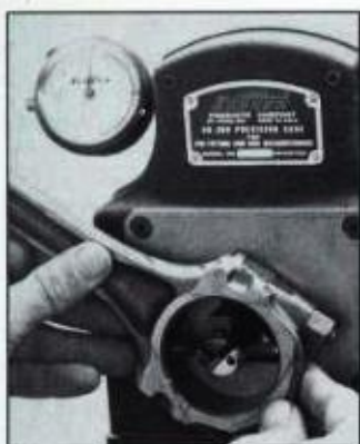
Mounted on rod honing machine, indicator is preset to specification with micrometers. Connecting rod is then rotated on mandrel to indicate big-end ID. Each indicator division represents 0.0001 in. (0.002mm), so small discrepancies can be found.
