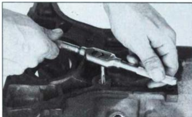
Clean threads with tap to ensure bolts are accurately torqued. Wire brush can be used to clean external threads, but you'll need the correct size and pitch taps for chasing threaded holes.
