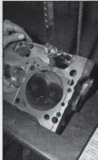
Volume of irregular "containers" such as combustion chambers is determined with liquid measured from chemist's burette. Low viscosity liquid such as kerosene is used to fill volume sealed with clear acrylic plate.
