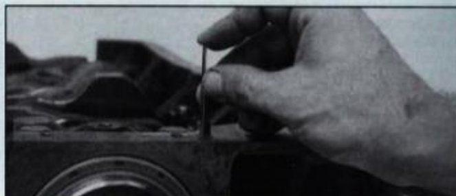
Rear main-cap seals are compressed in grooves by installing expander, a flat strip of metal with a chamfered end. Start expander in groove behind seal with sharp edge away from seal. Push expander into groove until it is flush with block. Note full-circle rear-main lip seal.
