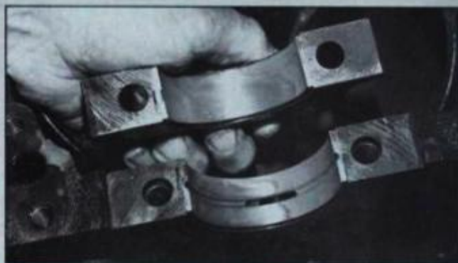
Main caps and bearings tell a story. If caps were loose in registers, chances are engine experienced severe detonation. Wear on grooved upper bearing half is more than on lower half of front insert because of upward force imposed by accessory-drive belts.
