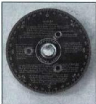
Available from camshaft manufacturers and high performance engine parts suppliers, a degree wheel is a must for checking camshaft against the manufacturer's specifications. Directions are printed on wheel.
