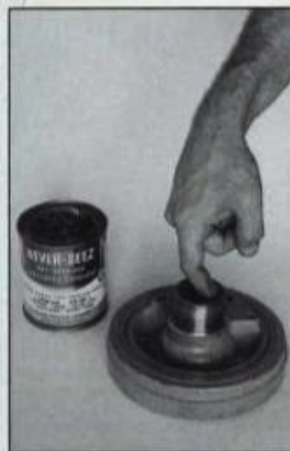
To ease installation and ease future removal, apply a thin coat of anti-seize compound to damper ID and oil-seal surface.
