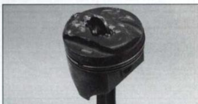
Burned piston at top was probably caused by pre-ignition, resulting in extreme blowby, low compression and power loss. At bottom, valve head imbedded itself in piston after breaking off at high rpm. Both conditions require engine teardown to correct.
