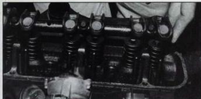
Install shaft-mounted rocker arms on head after all pushrods are in place. Apply high-pressure lube to valve tip and fit pushrods to rocker arms before you begin tightening hold-down bolts. Tighten bolts one turn at a time to keep from shaft.
