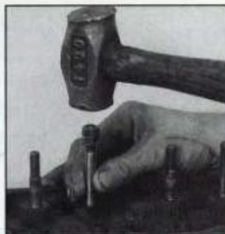
If original stud pulled out during engine operation or damaged one pulled out easy, ream for oversize stud. Ream should be 0.002-in. smaller than stud diameter. Thread on two nuts and jam them together. Run on top nut so it's flush with top of stud. Drive in stud with brass or lead mallet.
