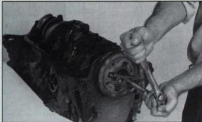
Damper is removed by pulling on bolts threaded into inboard portion of damper. Don't use gear puller to remove damper. It will pull off outer damper ring, rendering damper useless.
