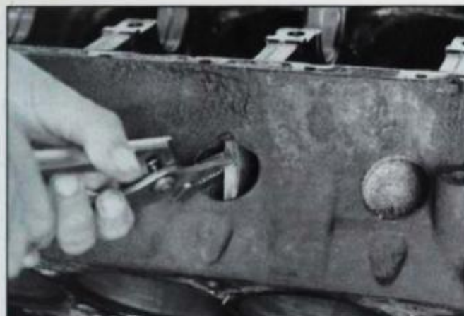
Use large dowel or punch to drive in core plug, grasp flange with pliers and lever plug out of core hole. Condition of core plugs indicate how well cooling system was maintained.
