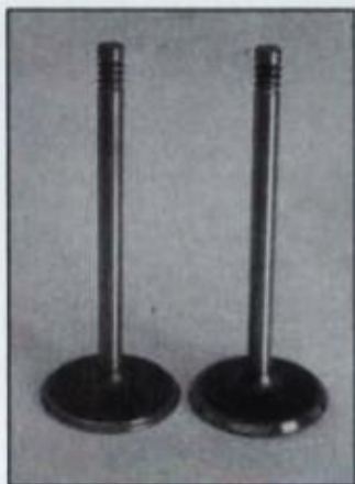
Lapped versus unlapped valve. Gray band on face should be full-circle to ensure sealing. If it's not, face is not concentric with stem and valve should be reground. Same goes for valve seat. If it's not full-circle, face is not centered on stem.
