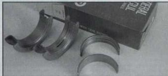
Wide flanges on one set of main bearing inserts resist crankshaft thrust loads as opposed to single-purpose radial bearing inserts at right. Holes and grooves in upper bearing halves are for lubrication.
