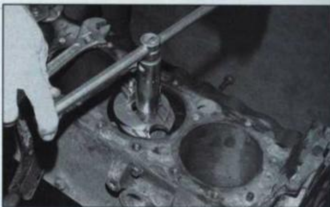
Removing ridge with ridge reamer. This will allow piston to come out top of bore without ring hanging up and damaging ring land. Removing ridge is a must if you intend to reuse pistons.
