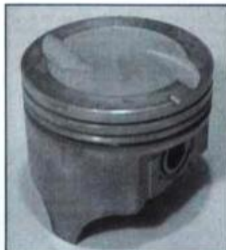
Shape of piston dome requires that piston is oriented correctly in bore to prevent piston-to-valve and cylinder head contact.
