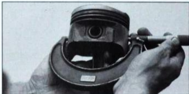
Measure piston diameter 90° to and level with bottom of wrist-pin bore. Measurement across bottom of skirt should be slightly more, or about 0.0005 in. (0.01mm)
