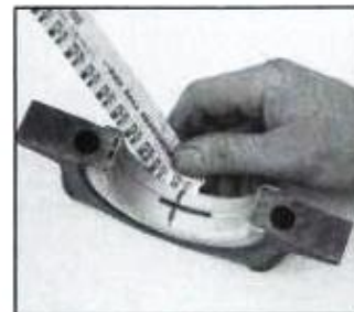
Double-check main bearing oil clearance with Plastigage. With crankshaft in place on dry bearings, lay strip of Plastigage the full length of the dry bearing journal, then install bearing cap. A very light film of oil can be applied to bearing in cap to keep Plastigage from sticking to bearing. Torque bolts to specification. Don't turn crankshaft. Carefully remove cap with bearings and check width of squeezed Plastigage with scale printed on edge of sleeve. Width corresponds directly to bearing oil clearance.
