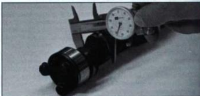
Lobe lift being measured with vernier calipers. Measure across base circle, then across heel and toe. Difference is gross lobe lift. Measurement is not accurate with high-performance cams as ramp areas extend too far around lobe, thus affecting reading.
