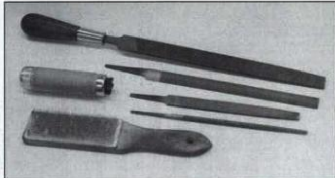
Assortment of files in cut and shape are used to smooth rough surfaces and break sharp edges. Handle installs on tang to make filing easier and safer; file card is for cleaning file teeth.
