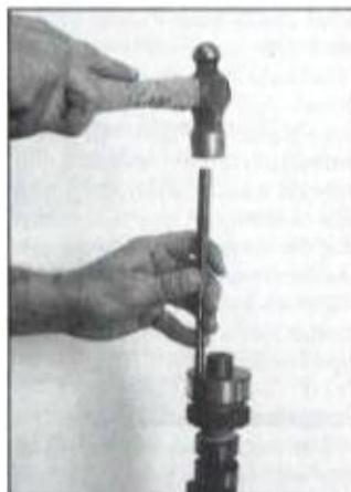
Rather than removing scar marks from drive pin, take advantage of them. Install scarred end of pin first. Drive it in with a punch and hammer until it bottoms.
