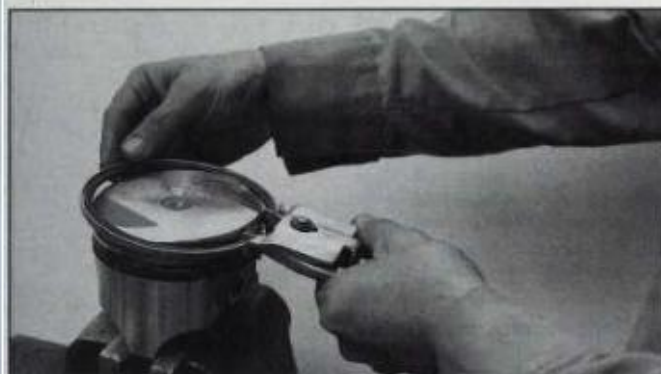
Install oil rings. Expander/spacer goes on first, then top rail followed by bottom rail. Check that expander/spacer ends butt rather than overlap. Don't spiral on compression rings. And rather than using your thumbs to expand them, use an expander. Place ring ends over groove, then rotate back of ring down over piston over and into groove.
