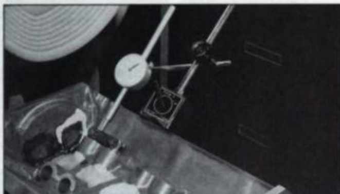
Most accurate way of measuring lobe lift is with dial indicator on lobe. Indicator is zeroed when lifter is on lobe base circle, then read as lobe lift when needle shows highest indicated reading as cam is rotated. Note link tying roller lifters together.
