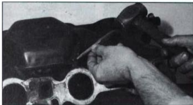
Don't overlook servicing bottom of intake manifold. If yours has a baffle attached to bottom it will have to come off so you can remove baked-on deposits. If rivets attach baffle, remove them by first raising each rivet slightly. Do this by lightly wedging small chisel under rivet head. This will allow you to clamp on rivet head with Vise Grip pliers. This done, carefully work out each rivet.
