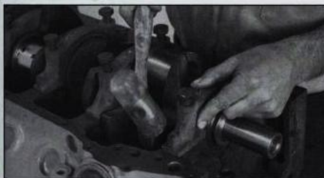
With bearings in place and oiled, install main bearing caps. A tap on side will seat cap in register. Don't force cap into place by tightening bearing cap bolts. You may damage block or cap. Double-check that caps are in the correct position and direction.
