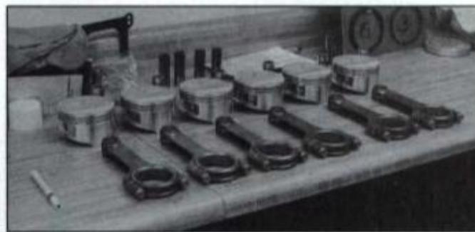
Pistons, pins, connecting rods and new Spiralox retainers are organized prior to assembly. Pin retainers should never be reused. Install new ones. Note board for organizing rings for V6 racing engine.
