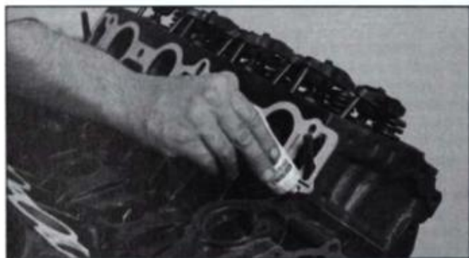
V-type engines use end gaskets between manifold and block. Due to difficulties in sealing, I prefer using a thick bead of RTV at both ends in place of gaskets.
