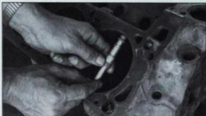
Requiring a special touch, inside micrometers are used for measuring inside diameters such as main bearing and cylinder bores. Extensions are used to change measuring ranges.
