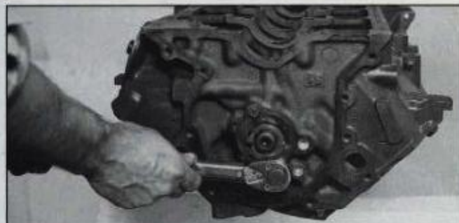
Once cam is in place, install thrust plate if engine is so equipped. Be careful to orient thrust plate correctly. Torque bolts to specification.
