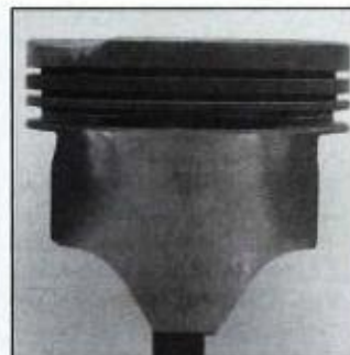
Wear pattern on skirt is straight and symmetrical. This indicates connecting rod is straight.
