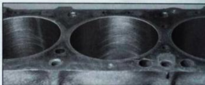
Cross-hatch pattern is particularly important if chrome-faced rings are to be used. Stroke speed and hone rpm determines cross-hatch angle, which should be between 20° and 60°.
