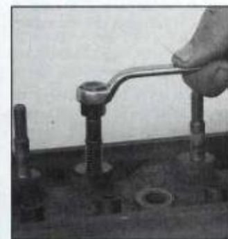
Standard threaded stud can be installed in place of pressed-in stud. Using a special tap, thread hole in stud boss. Tap has pilot so it follows hole during tapping to maintain stud alignment. Apply locking sealer to stud threads and run stud in with two nuts jammed together. Measure up from stud boss to place stud at same height as original studs.
