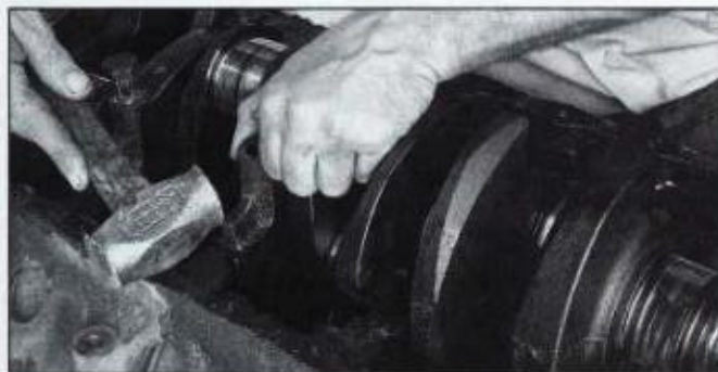
Once all pistons and rods are out, remove main-bearing caps. Check first that they are numbered. If not, number caps before you remove bolts. Once bolts are out, tap on side with soft mallet to free cap from register or dowels.
