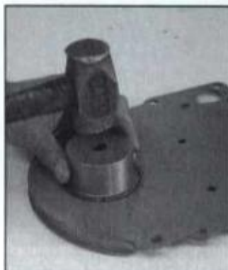
Apply grease or RTV to seal OD and position seal over bore in front cover. Seal lip should point toward engine side of cover. While cover is firmly supported on back side, drive seal in from other side. A large-diameter socket and brass hammer is used here.
