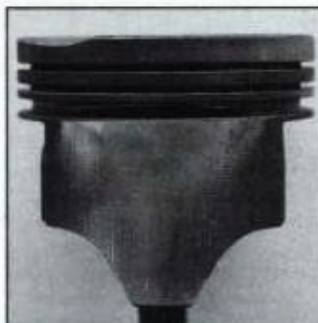
Skewed wear pattern on skirt indicates connecting rod is bent or twisted. Rod should be checked in fixture.
