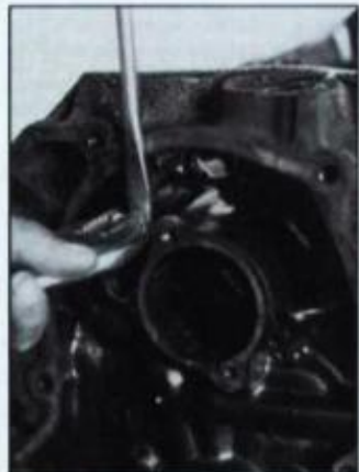
Once pipe plugs are out, drive out each cup-type plug with a long steel rod inserted into the oil gallery. Another option is to drill a small hole in each plug, thread a sheet-metal screw into plug, clamp onto it with Vise Grips and lever it out with a pry bar or large screwdriver.
