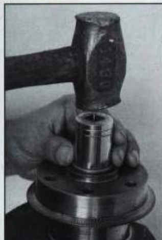
If used with manual transmissions, install pilot bearing. Drive pilot bushing or bearing in with hammer and hollow punch. If bearing is used, make sure punch seats against outside race only.
