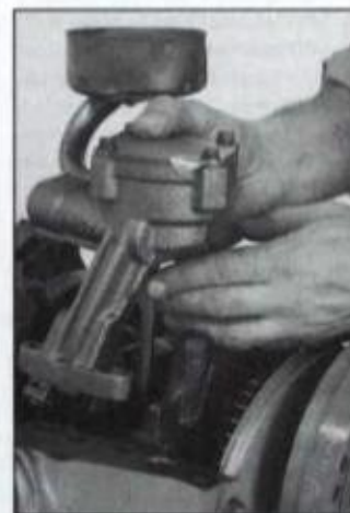
Install oil pump with driveshaft and gasket. Grease will help seal gasket and hold it in place. Don't use sealer on gasket.
