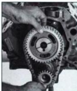
With chain hanging from cam sprocket and crankshaft sprocket laying in chain so timing marks align, fit crank sprocket to crankshaft nose. Engage keyway in crank sprocket with key in crankshaft, then cam sprocket with pin or key in cam. You may need to rotate crankshaft one way or the other a slight amount to align cam sprocket.
