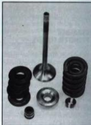
Valve, spring, Teflon seal and related hardware organized for installation into race head for Grand National NASCAR engine. Organization is important regardless of engine, be it for racing or the street. Titanium retainer and high-angle keepers are used. Spring assembly is made up of inner and outer valve springs with flat wound damper in between. Shims and seat install between spring and aluminum head.
