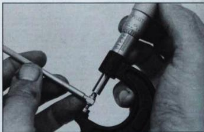
Telescoping gauges, commonly called snap gauges, must be used with outside micrometers for making inside measurements. Although relatively easy to use, you must practice with these transfer gauges in order to get accurate readings.
