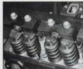
For high performance applications, stud girdle supports individual rocker-arm studs. Adjust valves, then fit girdle loosely to stud extensions. Gradually tighten securing nuts to manufacturer's specs. A "tall" valve cover will be needed to allow room for girdle.
