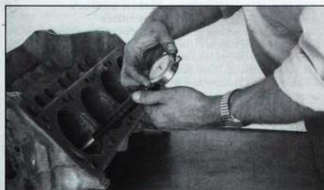
Dial bore gauge is used to measure bore wear directly. Typically maximum wear is found immediately below ridge in line with main-bearing bores in end cylinders and 90° to mains for all others. Check several other positions to make sure, though.
