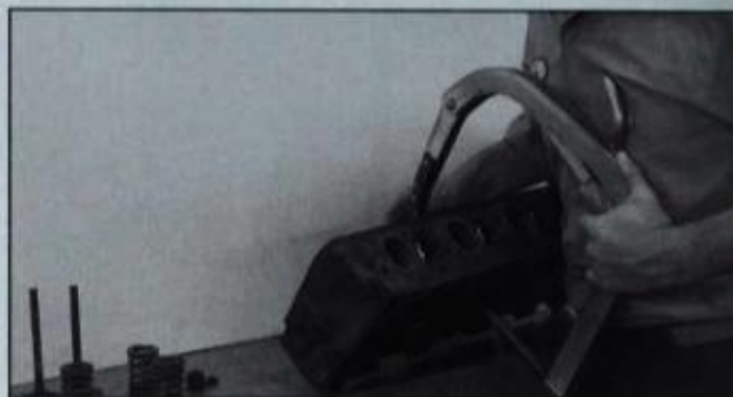
After breaking loose retainers, compress valve spring just enough to allow removal of keepers. You'll need a valve spring compressor to do this.
