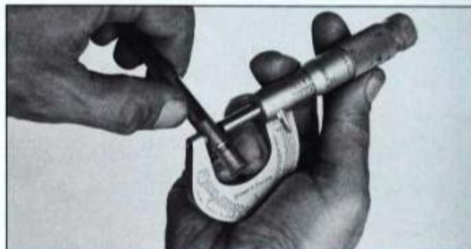
Using a 1-inch micrometer, compare measurements taken from an unworn section of valve stem and that having maximum wear. The difference between these two measurements is stem wear.
