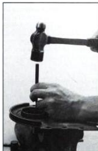
Carefully remove lip seal from front cover. Aluminum covers are easily broken and sheet-metal covers are easily bent. Use a hook-type seal remover or punch and hammer and work seal out a little at a time.
