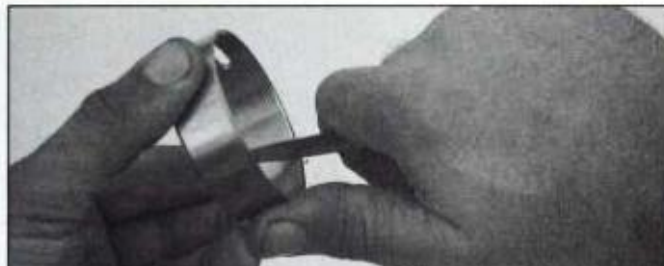
New cam bearings have square or ragged edges. To ease cam installation, chamfer edges of bearings with a pocket knife or bearing scraper before you install them.
