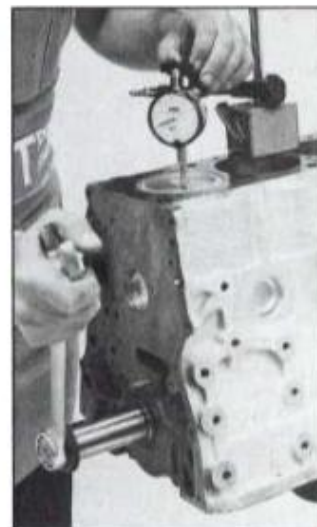
One method used to find TDC is with dial indicator on piston and a wrench to turn crankshaft. Although not yet installed, bolt degree wheel to crank nose and attach pointer to front face of block. As piston passes TDC, indicator pointer reaches maximum and swings back in other direction. Trick is to have pointer indicate 0 the instant it reverses direction.
