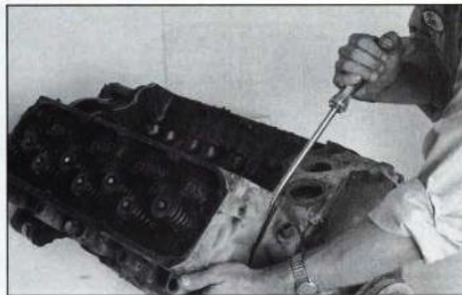
Except for two loosely installed bolts, make sure all head bolts are removed before you try to break head loose from block. Lever off head with breaker bar inserted into intake port; use block of wood with aluminum heads. Take care not to damage gasket surface if you wedge between block and head.
