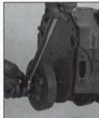
Install with washer and torque damper bolt. To keep crankshaft from turning use a large screwdriver between block and crank counterweight. If oil pan is in place, use two bolts in damper or flywheel flange and bridge them with a screwdriver or pry bar.
