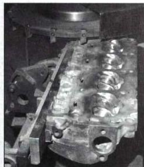
Complete cylinder head reconditioning by giving gasket surface a light cut on milling machine. Note polished combustion chambers, which was part of porting job. Cylinder head was tested on flow bench to ensure modifications increased port flow.
