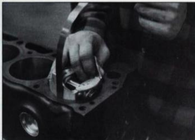
Ribbon gauge is a specialized feeler gauge for measuring piston-to-bore clearances. Gauge and piston are inserted into bore, then ribbon gauge is pulled out with a fish type scale or by someone with a good feel. Pulling tension must be within specified range if clearance is within spec.
