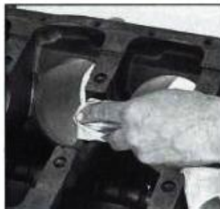
Before installing bearings, clean bearing bore in block and cap. Wipe back side of each bearing insert too and fit inserts into block and caps.
