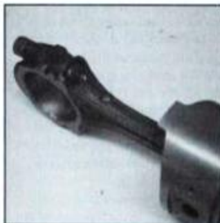
Some connecting rods have an oil hole in beam for lubricating thrust-side of cylinder wall; others a groove in bearing-cap parting line. Because of this and a chamfer on one side of big end needed to clear bearing-journal radius for rods sharing one journal, connecting rods must be oriented correctly to pistons.
