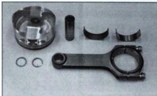
Disassembled connecting rod and piston. Full-floating wrist pin is held in place with Spiralox-type retainers. Pressed pins are held in place by an interference fit between small end of rod and pin.
