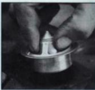
Install thermostat in the right direction. Flange fits in recess in block or manifold.
