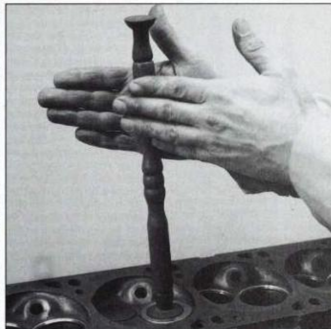
Lapping a valve starts by coating valve face with lapping paste. Valve is then installed on its seat and oscillated with light pressure using a lapping stick between the palms of your hands. Valves should be installed on the seats they were lapped on, so keep them organized.
