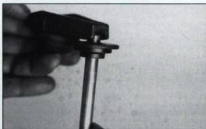
Infamous rail rocker arm, flanges on rocker arm straddle valve tip to stabilize rocker arm. If yours is this type, you can't recondition them. Replace them.
