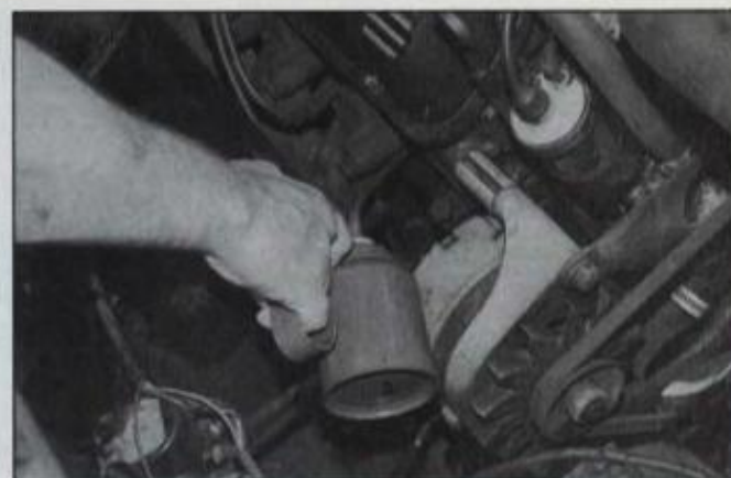
To isolate problem in weak cylinder, squirt a teaspoon of oil through spark plug hole and spin engine a few revolutions to distribute oil. Recheck compression. If compression improves, problem is ring-to-bore sealing; if it doesn't, problem may be a leaky valve or head gasket. Bad cam lobe or hole in piston is also a possibility.
