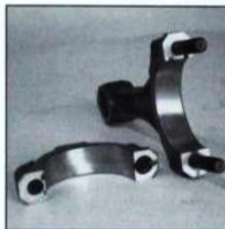
Some connecting rods have an oil hole in beam for lubricating thrust-side of cylinder wall; others a groove in bearing-cap parting line. Because of this and a chamfer on one side of big end needed to clear bearing-journal radius for rods sharing one journal, connecting rods must be oriented correctly to pistons.
