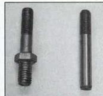
High performance screw-in rocker-arm stud compared to pressed-in stud. To convert from pressed-in to screw-in studs, stud bosses must be milled and stud holes tapped.
