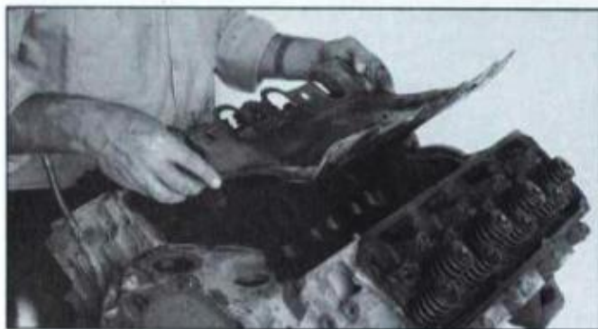
Some manifolds that seal top of block incorporate manifold-to-head gaskets with a baffle. If your manifold doesn't seal top of block, a separate baffle will be used. Remove it.
