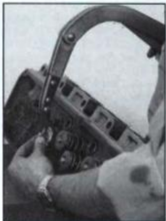
Compressing spring no more than necessary. Install keepers. Grease on keepers will hold them in place while you release compressor. Using soft mallet, tap valve stem tip to check that retainers are firmly seated in grooves.
