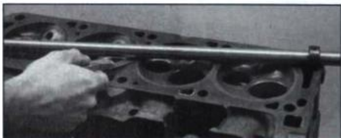
Check head surface flatness with a precision straight edge and feeler gauge. If 0.004-in. (0.10mm) feeler gauge fits under bar, head should be resurfaced. For an inline six and eight, make it 0.006 in. (0.15mm) and 0.008 in. (0.20mm), respectively.
