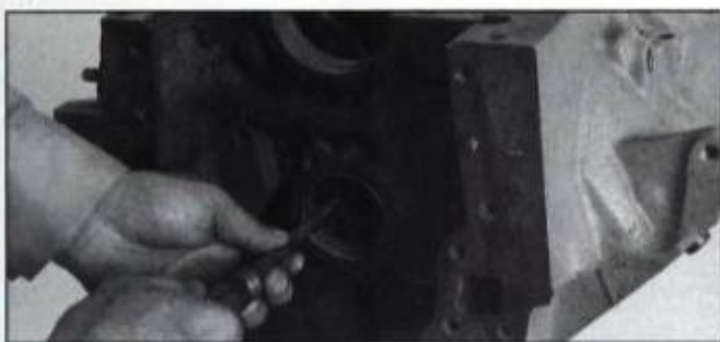
Bluing and scraping cam bearings is what you'll have to do if cam is tight in the new bearings. I'm doing front one here. Center bearings are harder to do because of accessibility. This job is for an expert.
