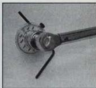
Some bolts used in modern engines, particularly head bolts, are torqued to a specific value, then rotated through a specified angle such as 50°. To do this accurately, you'll need an angle gauge.
