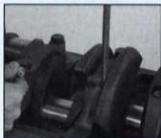
Two ways of checking crankshaft end play; with dial indicator and feeler gauges. With dial indicator, force crankshaft to rear of block using a screwdriver. Hold it there, zero the dial indicator and force crankshaft forward. Read end play directly. Using feeler gauges, hold crankshaft in one direction while you measure clearance between bearing and crankshaft thrust face.
