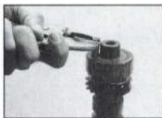
New camshafts sometimes don't come with a drive pin. If this is the case, remove pin from your old camshaft before you turn it in as a core. Remove pin by clamping on it with Vise Grips and work it out.
