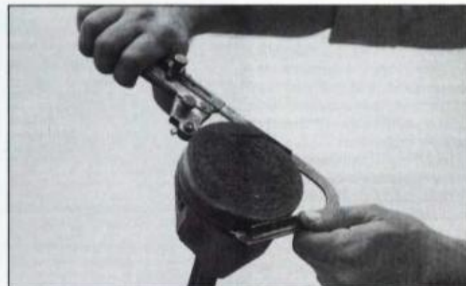
Adjust ring groove cleaner to groove width and diameter, then run tool around groove to remove carbon deposits. Be careful not to remove metal.
