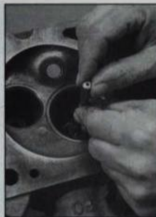
Direct measurement is the best way of determining valve guide wear. Small-hole gauge is first expanded to fit largest section of guide, then it is miked. If valve stem diameter subtracted from this figure is more than 0.002 in. (0.05mm), guides should be reconditioned.
