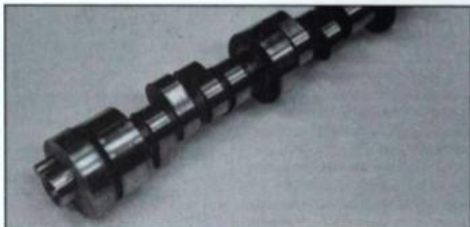
Unlike flat-tappet cam that uses tapered lobes, roller cam-lobe surfaces are parallel with centerline of cam. Another difference: roller cam is machined from steel billet rather than cast iron.
