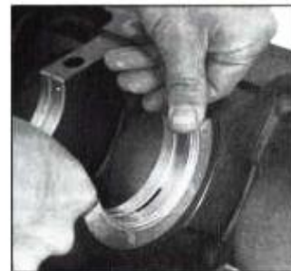
Before installing bearings, clean bearing bore in block and cap. Wipe back side of each bearing insert too and fit inserts into block and caps.
