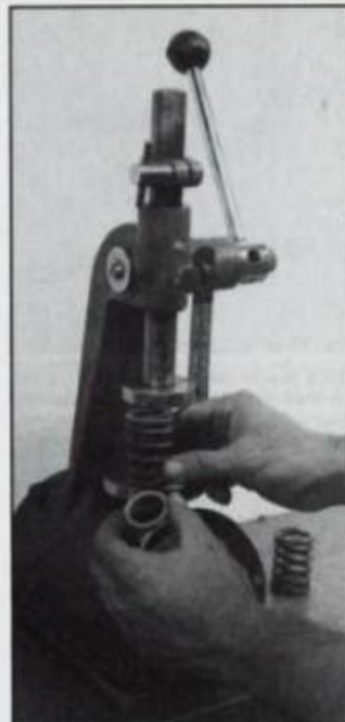
Checking spring load at installed height. Adding shims can be used to bring load within specification, but coil clearance should be checked with spring on shims at open height to assure it doesn't bind, or go solid. There should be at least 0.060 in. (1.5mm) between coils. You have a choice of 0.015-in., 0.030-in. and 0.060-in. shims.
