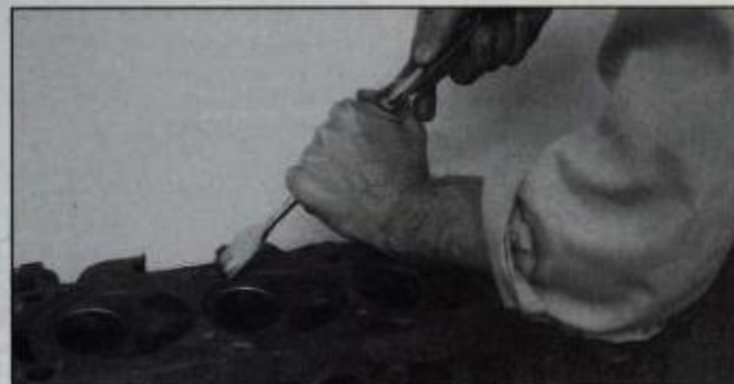
To ensure sealing, head gasket and other gasket surfaces must be clean down to bare metal. Be careful when scraping aluminum cylinder heads. Use chemical gasket remover and plastic scraper on aluminum. A large flat file is used to smooth over imperfections and remove small bits of gasket material.
