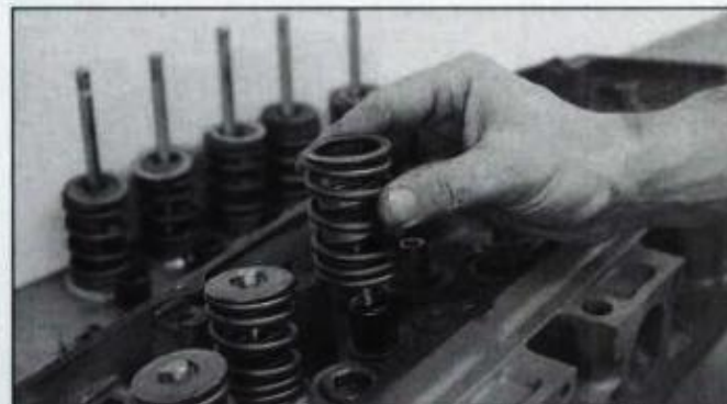
Spring seats and/or shims. If used, are installed between spring and cylinder head. In some cases, a shim or seat won't fit over the valve stem seal, so place them on spring pad before you install seal. Once seal, seat and/or shim are in place, install spring(s).
