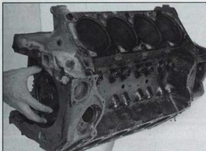
Before cam can be removed, lifters must be raised in bores so lobes will clear lifters. Do this by rotating camshaft at least one complete revolution. If used, thrust plate must come off to remove cam.
