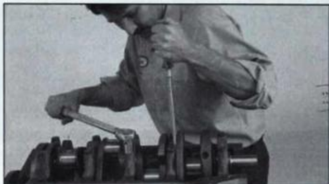
Torque cap with thrust bearing after seating bearing. Do this by forcing crankshaft back and forth with screwdrivers or pry bars between main-bearing webs and crank throws. Hold crankshaft forward, then tighten bolts.
