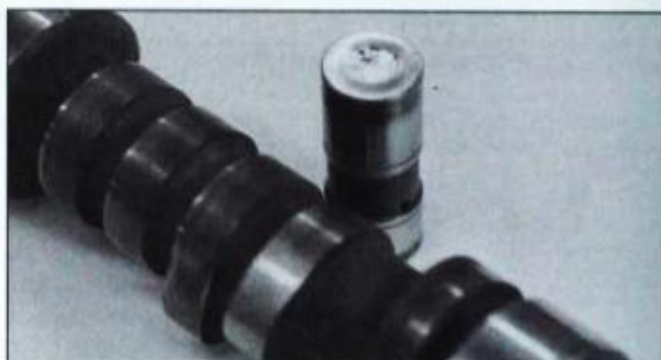
Lubes and lifters wear together. All it takes is for one lobe of a camshaft to be worn excessively to require replacement. Save cam, though. It may be OK as a core.
