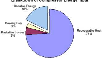
Breakdown of Compressor Energy Input
