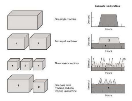
It is usually more efficient to run a small compressor at full load as opposed to a large one at low load.
